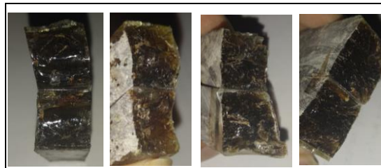
Gambar 4.3 Permukaan Patahan hasil Pengujian Bending 15%, 25%, 35%, 45%
