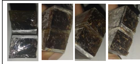
Gambar 4.5 Permukaan Patahan hasil Pengujian Bending 15%, 25%, 35%, 45%
