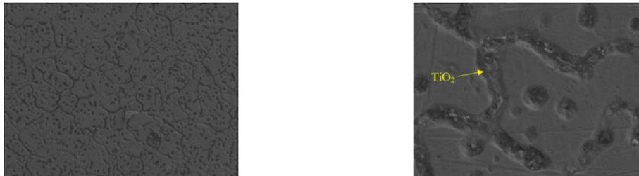
Gambar 9 Hasil FESEM micrograph pengelasan Aluminium paduan 3003 (a) 3% TiO<sub>2</sub>, (b) perbesaran gambar (a). [15]
