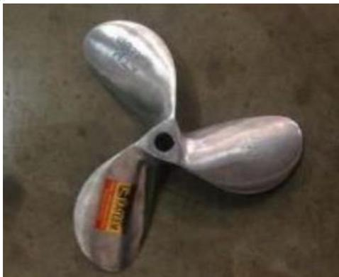
**Gambar 4.** Fixed Pitch Propellers berdaun 3 [3]
