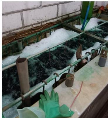
**Gambar 1.** Bak Elektroplating
