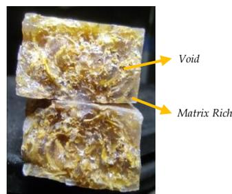
**Gambar 3** Hasil Patahan Spesimen A (X1, Y1, Dan Z1)
