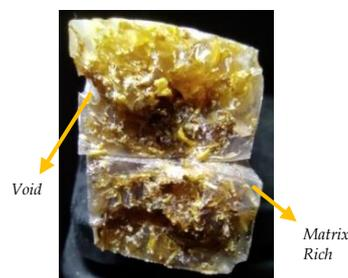
**Gambar 5** Hasil Patahan Spesimen C (X2, Y1, Dan Z2)
