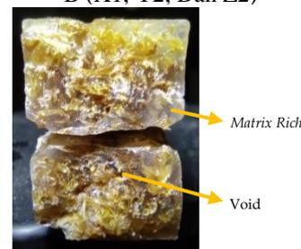
**Gambar 6** Hasil Patahan Spesimen D (X2, Y2, Dan Z1)
