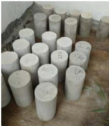
Gambar 7. Benda Uji Silinder 10 cm x 20 cm
